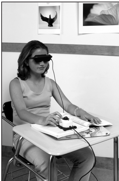
Figure 4-4. The Max™ can be used at work or school. With the viewing spectacles, no monitor is necessary. (Photo courtesy of Enhanced Vision, Huntington Beach, CA.)
